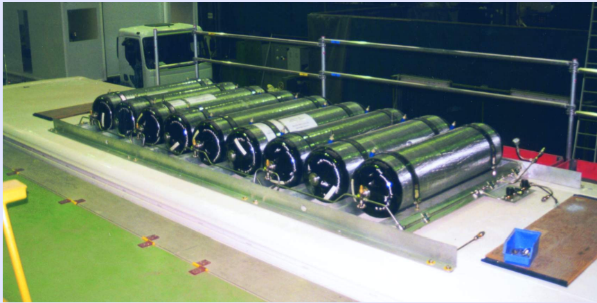
Roof top mounting of cylinders on a bus
