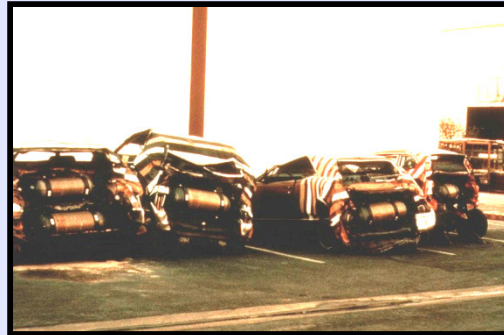
10 ...17....23...30m drops ...no leakage!!
