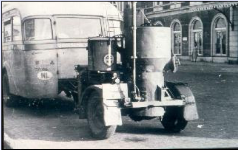
Bus with Coal Gasifier
